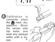
Note: A binking a mark indicates that the unit is not calibrated. Check that the correct standard solution was used and calibrate
